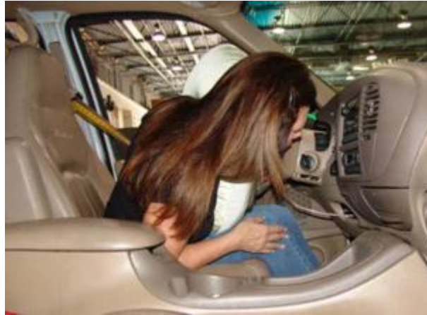
Figure 2. Out-of-position surrogate demonstrating how head can bypass inflated airbag during frontal impact
